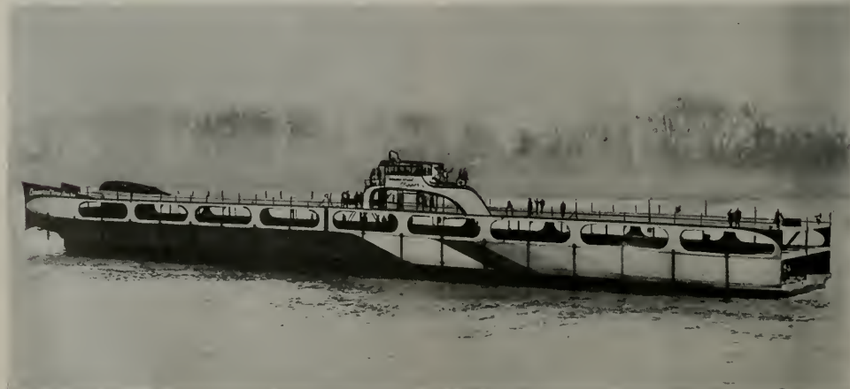
The Commercial Clipper operating with two of its three units during trial runs on the Mississippi. The center unit had not been completed at the time of the trials.
